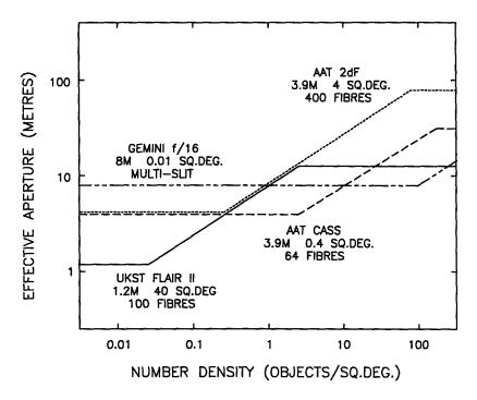
Figure 1. Effective aperture of four multi-object spectroscopy systems plotted against target object number-density.
