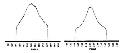
Figure 3. Output end intensity patterns when a  $153 \mu m$  diameter fibre is centrally illuminated at its input end by a spot of about 1/3 its diameter (left) and 1/10 its diameter (right), showing highly-incomplete scrambling. Beam focal ratio f/2.8.
