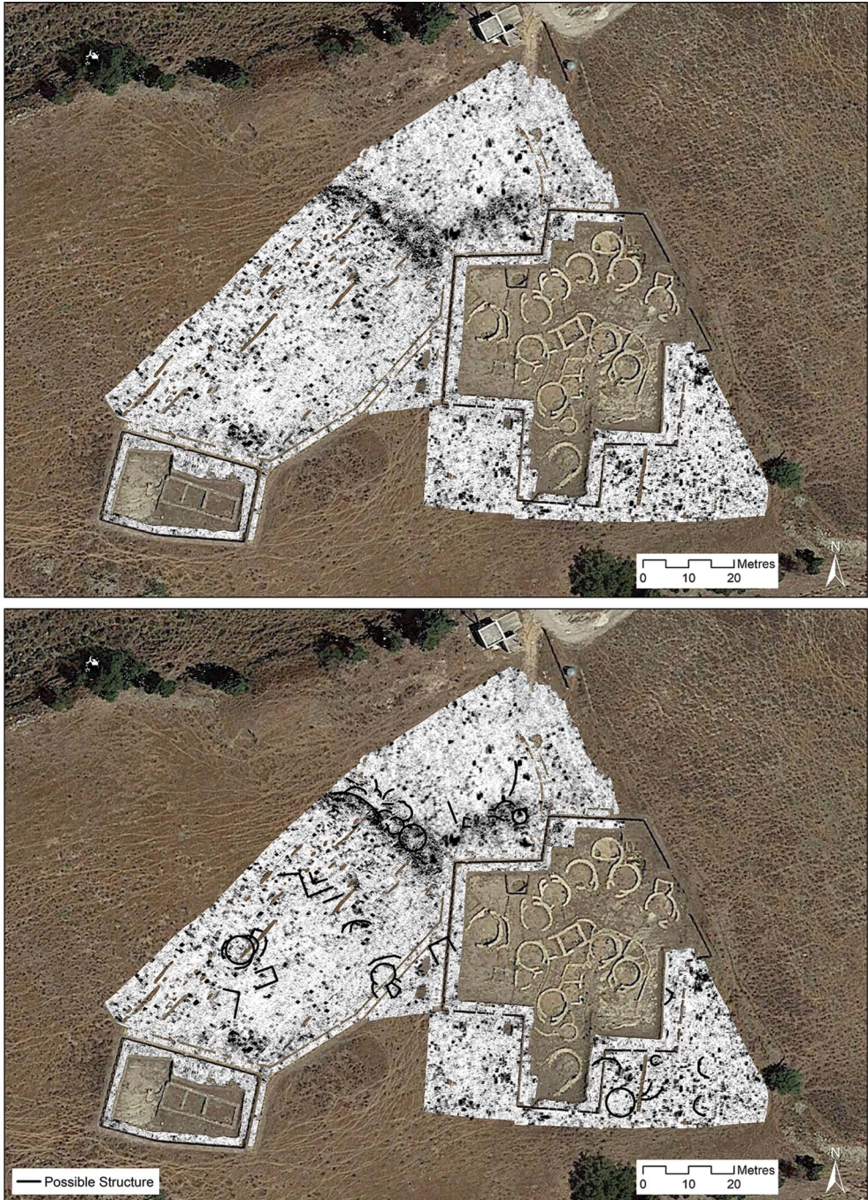
Figure 6. Top) GPR depth slice, 1–1.05m below the ground surface; bottom) interpretation of the anomalies seen in the GPR data (background images © Google Earth 2016; figure by the authors).
