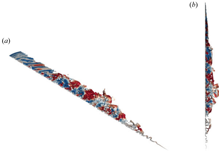
Figure 10. Vortical flow structures visualised by the iso-surface \lambda_2 = -0.001 coloured by w/(\Omega R) at \Omega t = 50 rad for Re = 1.5 \times 10^5 . The colour is consistent with figure 2(c), where the dimensionless axial velocity w/(\Omega R) ranges from -0.005 (blue) to 0.005 (red).
