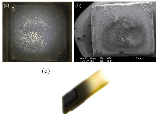
**Fig. 12.** (Color online) Surface observation of contact at 100 Hz. (a) Optical microscope [zoom:75], (b) SEM, (c) image of contact and its electrode support.
