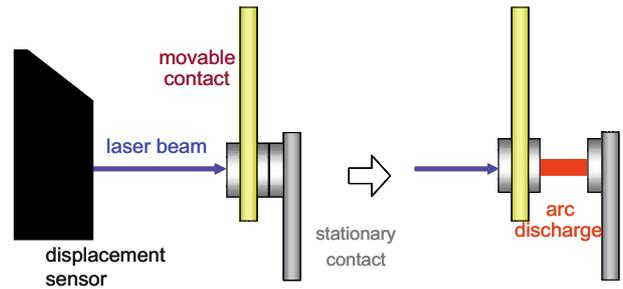
Fig. 4. (Color online) Measurement of separating speed (Left: ON state, Right: OFF state).
