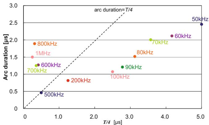
**Fig. 9.** (Color online) Relationship between arc duration and  $T/4$  (from 50 kHz to 1 MHz).
