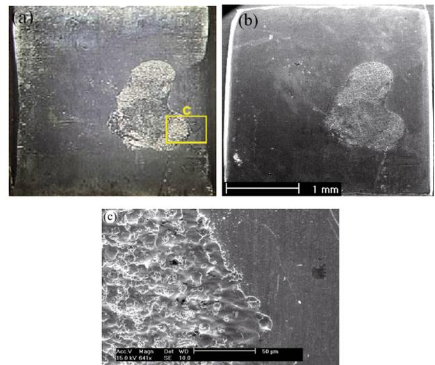
**Fig. 17.** (Color online) Surface observation of contact at 500 kHz. (a) Optical microscope [zoom:75], (b) SEM, (c) magnified view of square of (a).
