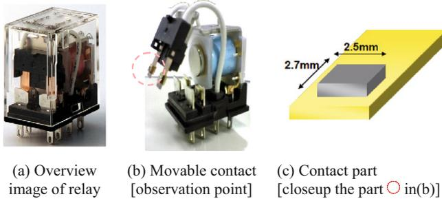
Fig. 2. (Color online) Relay used in this experiment.
