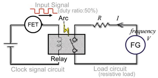
Fig. 3. (Color online) Experimental apparatus of the switching experiment.
