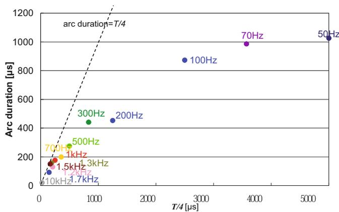
Fig. 7. (Color online) Relationship between arc duration and  $T/4$  [from 50 Hz to 10 kHz].
