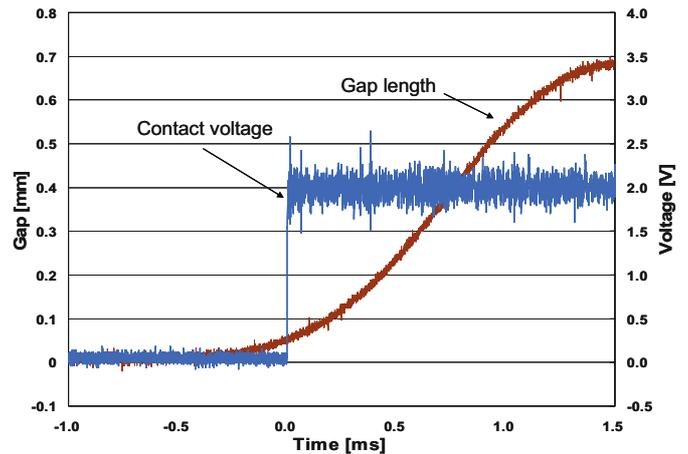
Fig. 5. (Color online) Gap length and voltage between contacts at dc power.
