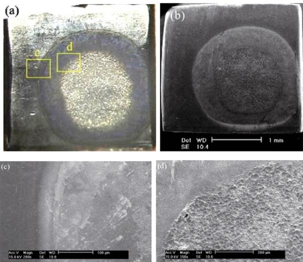
**Fig. 14.** (Color online) Surface observation of contact at 10 kHz. (a) Optical microscope [zoom:75], (b) SEM, (c, d) magnified view of square of (a).
