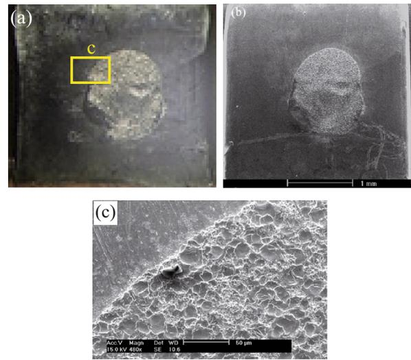
**Fig. 16.** (Color online) Surface observation of contact at 100 kHz. (a) Optical microscope [zoom:75], (b) SEM, (c) magnified view of square of (a).
