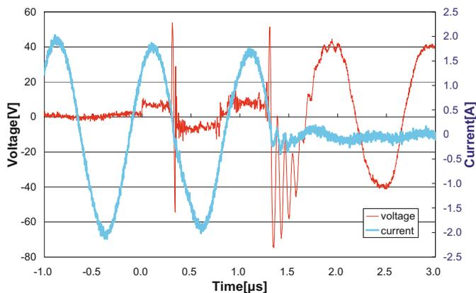
**Fig. 10.** (Color online) Re-ignition waveform at 1 MHz.
