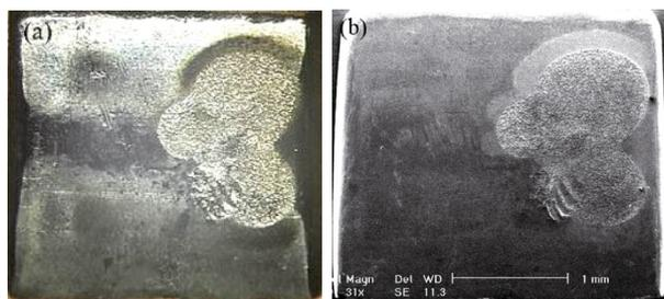
**Fig. 15.** (Color online) Surface observation of contact at 50 kHz. (a) Optical microscope [zoom:75], (b) SEM.
