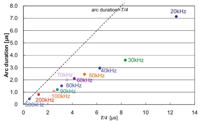
Fig. 8. (Color online) Relationship between arc duration and  $T/4$  [from 20 kHz to 500 kHz].
