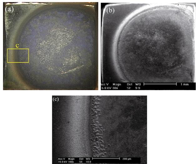
**Fig. 13.** (Color online) Surface observation of contact at 1 kHz. (a) Optical microscope [zoom:75], (b) SEM, (c) magnified view of square of (a).
