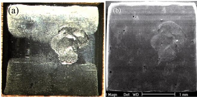
**Fig. 18.** (Color online) Surface observation of contact at 1 MHz. (a) Optical microscope [zoom:75], (b) SEM.
