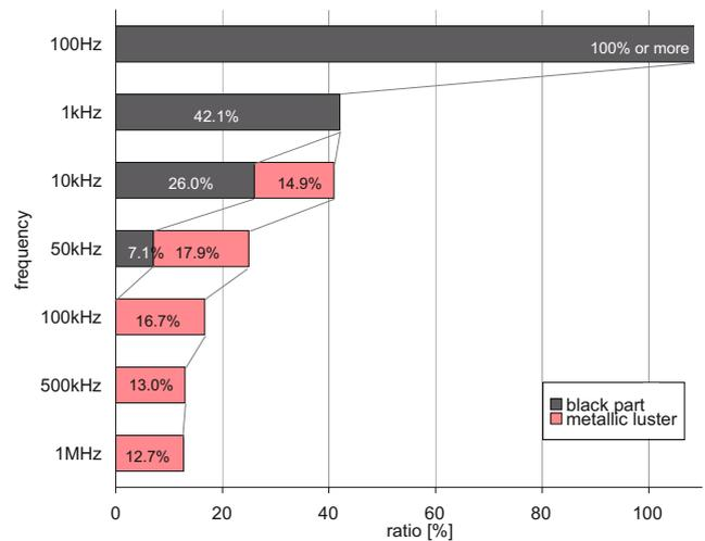
**Fig. 19.** (Color online) Proportion of the damage by arc to whole contact area.
