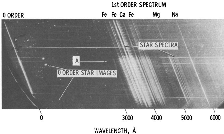
FIGURE 2.—Enlargement of a spectrogram of a Taurid meteor.
