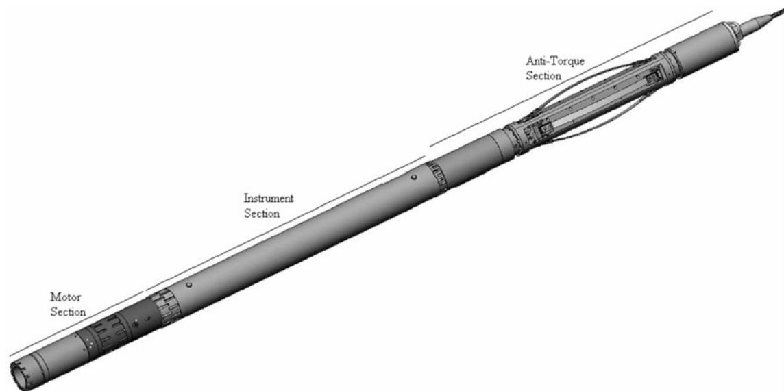
**Fig. 3.** Upper sonde. Though shown in isometric view, the sonde normally hangs vertically in the borehole on its cable. The cable attachment can be seen in the upper right corner. Most of the upper sonde does not rotate. The bottom half of the motor section rotates, providing the rotation needed for the cutting action.
