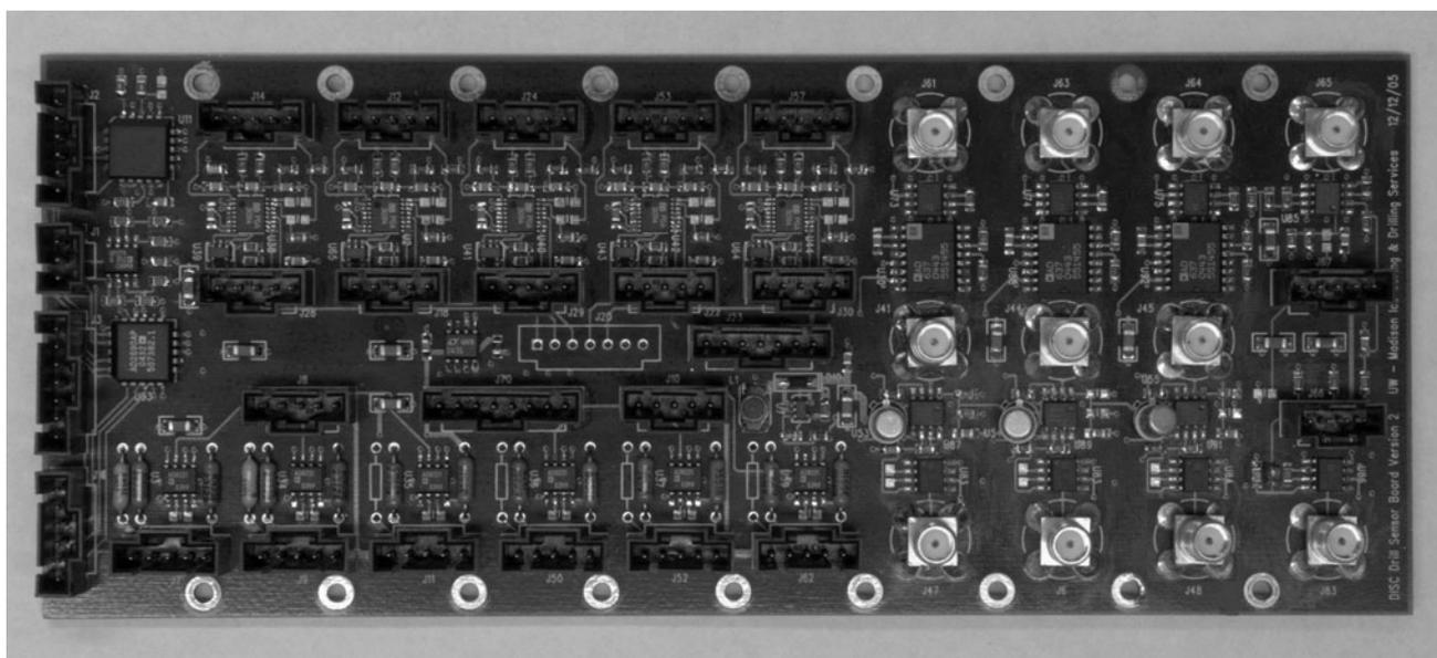
**Fig. 5.** Sensor board. A large number of connectors are used to connect the sensor board's conditioning electronics to the individual sensors. Additional connectors transfer the conditioned analog signals to the on-board computers.
