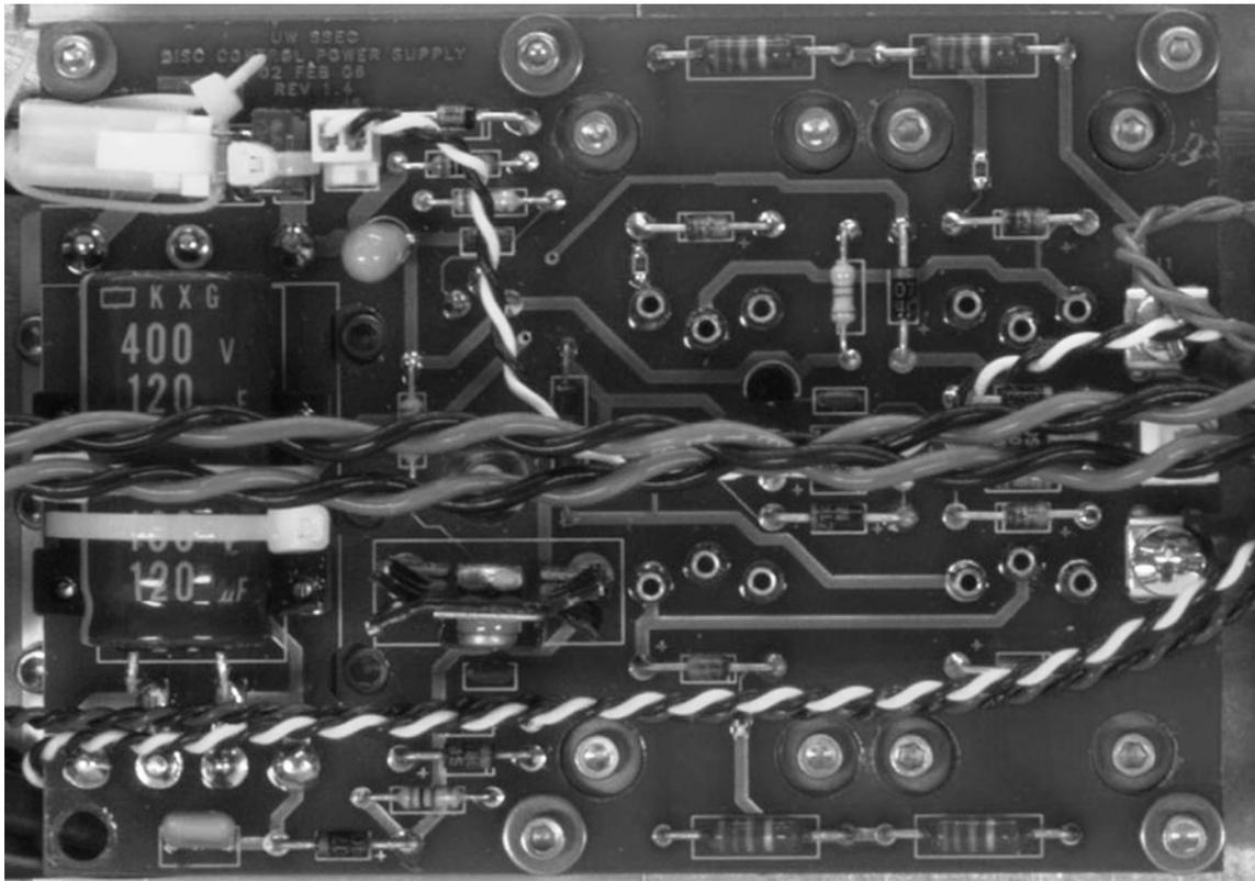
**Fig. 9.** Control power supply. The CPS is implemented using a simple linear regulator (note the low amount of components on the circuit board). The pass element of the linear regulator is implemented using MOSFETs located between the circuit board and the base plate. The size of these large components determines the overall size of the CPS.
