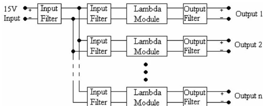
**Fig. 10.** Block diagram of LVPS design. The use of off-the-shelf power modules enables a simple design strategy. The same basic design is simply repeated for each required output. Not shown is the isolation barrier between the input 15 V rail and each output rail. The output rails are also generally isolated from each other.
