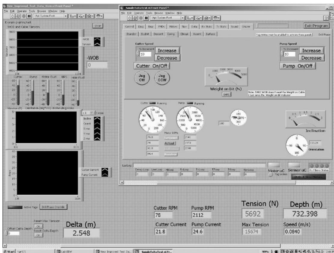
**Fig. 2.** Sonde control screen. A multitude of indicators present cutter speed, pump speed, temperatures, etc., to the operator. Motor speeds can be set by entering desired rpm into data fields. Real-time graphs are used to display critical data (motor torques, WOB, etc.).
