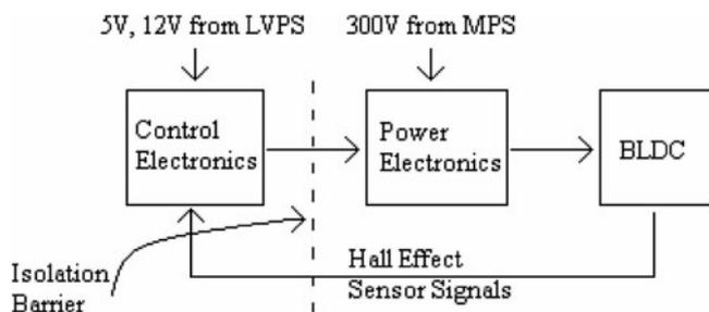
**Fig. 4.** Block diagram of motor-driver architecture. Control electronics govern a power stage which, in turn, drives the BLDC motor. Velocity feedback is achieved using Hall-effect sensor signals. The Hall-effect sensors also provide commutation information. An isolation barrier protects the control electronics and other associated electronics from over-voltage in the event of a motor failure.
