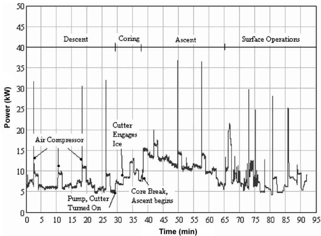
**Fig. 13.** Power consumption during a drill run. Power consumption is low during descent, climbs during ascent and becomes erratic during surface operations where various machines are used. Tripping speeds were  $0.5 \text{ m s}^{-1}$  during this drill run.
