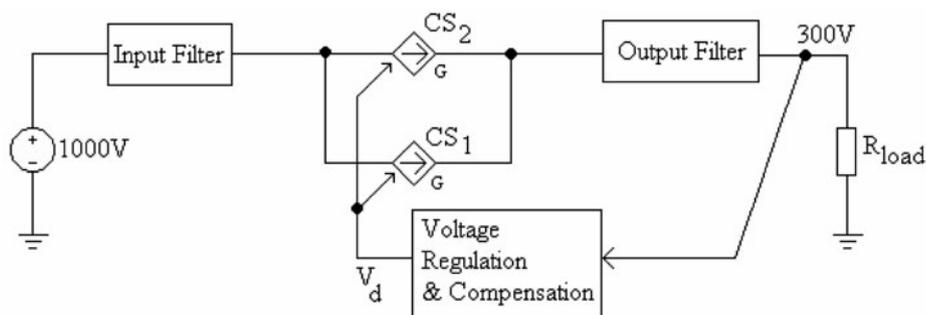
**Fig. 7.** Simplified MPS operating principle. Two voltage-controlled current sources are operated in parallel. A voltage loop ensures constant output voltage over the load range of 0–5 kW. Input and output filters provide low-noise power buses.
