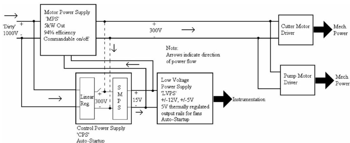
**Fig. 6.** Power system architecture. Automated start-up capability allows for the system to power up automatically as soon as 1000 V power is applied. As a safety feature, the MPS requires a separate control signal from the surface computer to start.
