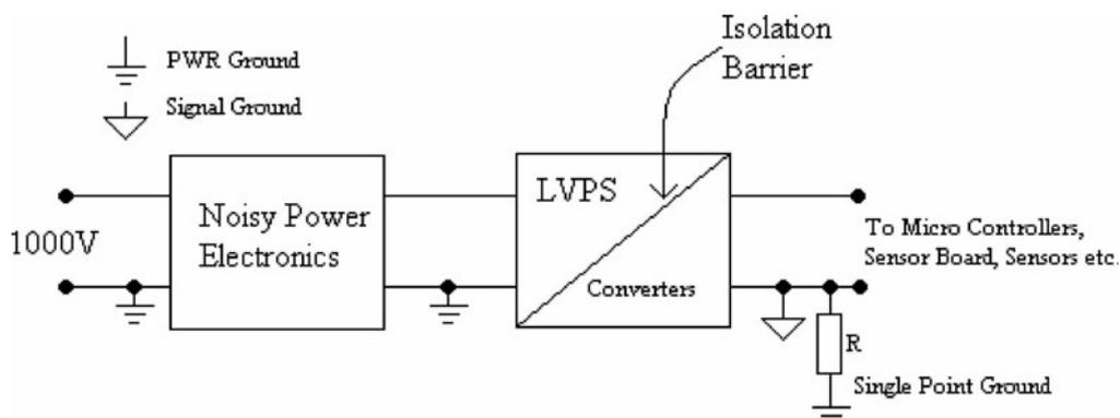
**Fig. 12.** Single-point grounding. Signal ground connects to power ground at one point only, through resistor R. This allows the noise currents from noisy members of the system to be steered away from the sensitive low-noise electronics.
