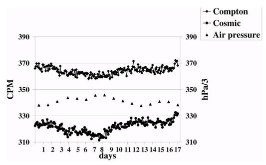
Figure 1 Guard Compton electron and muon peak count rate variation with air pressure on the surface (Wallac low-level laboratory) for 17 days. Air pressure reading (hPa) has been divided by 3 to scale down.
