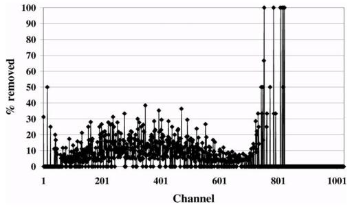
Figure 5 Guard efficiency in the Gran Sasso National Laboratory measured with a water sample, 8 mL:12 mL (water: Ultima Gold LLT)
