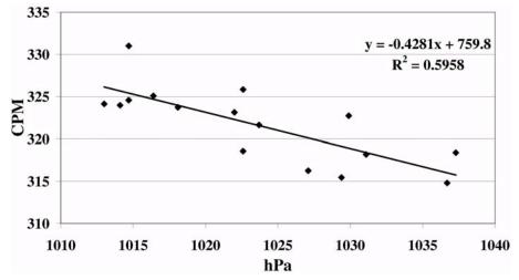
Figure 2 Guard muon count rate versus atmospheric pressure
