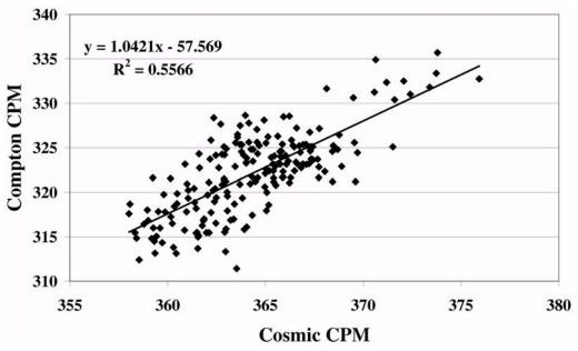
Figure 3 Compton count rate versus cosmic muon count rate under variable air pressure for 17 days
