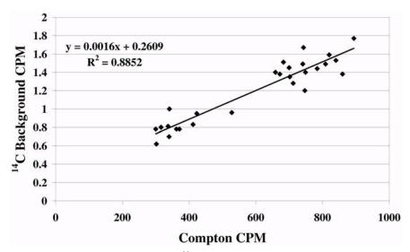
Figure 6 Background count rate in optimum <sup>14</sup>C window versus guard Compton rate in 15-mL copperteflon vials in 27 laboratories. Sample is benzene with 15 mg/mL butyl-PBD as scintillant.
