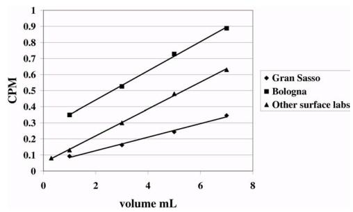
Figure 7 Background dependence on benzene volume in Gran Sasso National Laboratory, 9-mL unmasked teflon vial (CPM =  $0.0422 \times V + 0.0422$ ); Radiocarbon Laboratory ENEA-Bologna, 9-mL teflon vial (CPM =  $0.0908 \times V + 0.2598$ ); other surface laboratories, 3-, 7-, 15-, and 20-mL masked copper-teflon vials and 0.3-mL teflon vial in a black masking Delrin adapter (CPM =  $0.0844 \times V + 0.0507$ ).
