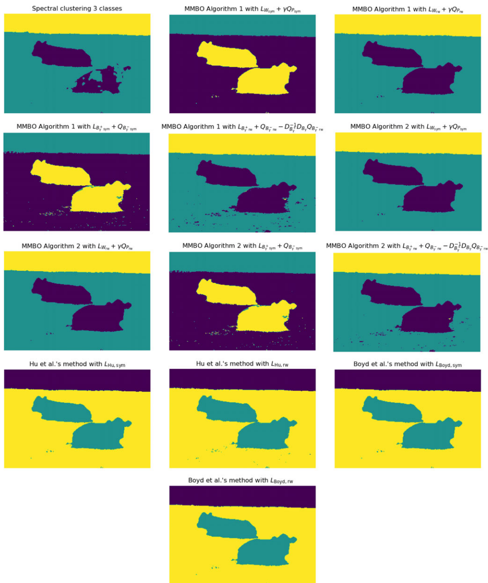
Figure 8. The ‘two cows’ image is segmented using different methods with \gamma = 1 . The number of clusters K used by MMBO algorithms, Hu et al.’s method and Boyd et al.’s method is obtained from the ground truth (shown in Figure 7), that is, K = 3 . Moreover, for the MMBO scheme, Hu et al.’s method and Boyd et al.’s method, we choose m = K = 3 . Each method’s displayed image segmentation result is the one with the highest modularity scores for that method from among 20 runs.
