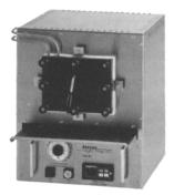
**Gastight Muffle Furnace.** Fibre insulated muffle furnace with heat resistant gastight muffle insert for inert gas operation up to 1100 °C. Water cooled door flange. Chamber volume up to 200 liters available, based on our KS-series. As an option vacuumtight for temperatures up to 800 °C, gas supply, exhaust with burner.
