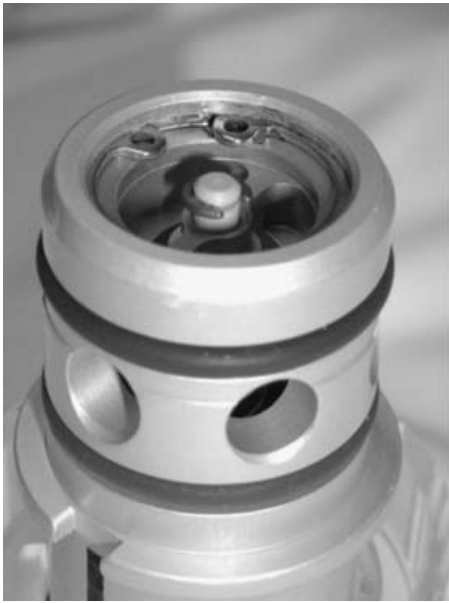
Figure 1. Visible rust on the lower end of the adjustable pressure limit valve, which led to an intermittent blockage of the valve. The loss of the gas-release ability caused an excessive build-up of the gas pressure in the breathing circuit.
