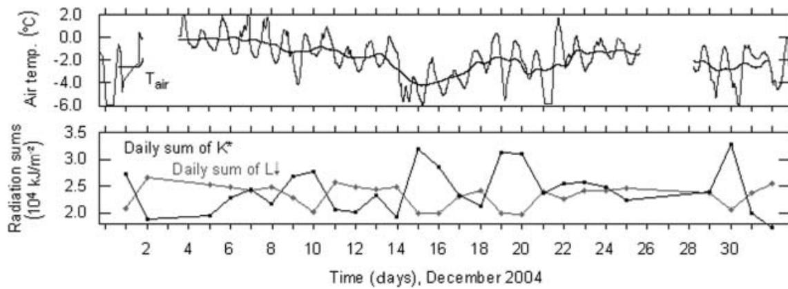
**Fig. 4.** Time series of air temperature ( $T_{air}$ ), daily mean  $T_{air}$ , daily sum of global radiation ( $K^*$ ) and daily sum of longwave downward radiation ( $L_{\downarrow}$ ) as measured by the AWS on the ISPOL floe, December 2004. Measurement gaps are due to rescues of the AWS when the floe broke up.
