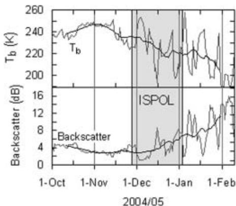
**Fig. 2.** Time series of daily mean SSM/I brightness temperature (37V) and QuikSCAT backscatter coefficient (13.4 GHz) at the ISPOL position, 1 October 2004 to 10 February 2005. Black lines represent 21 day moving averages. The period with coincident in situ measurements during ISPOL is highlighted by a grey box (cf. Fig. 1).
