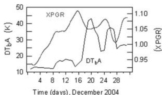
**Fig. 6.** Time series of the XPGR parameter (19H/37V, 3 day moving average) and the diurnal  $T_b$  amplitude from SSM/I swath data ( $DT_{bA}$ , 3 day moving average), December 2004.
