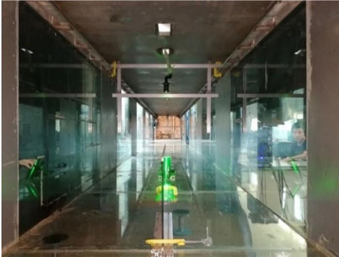
Figure 1. Working section of the wind tunnel taken from the inside.
