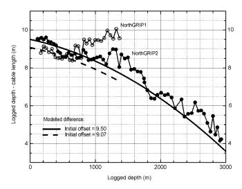
Fig. 2. Comparison between the logged depth and the unwound cable length. Data are plotted for approximately every 15th run for NorthGRIP 1 (thin line/open circles) and for North-GRIP 2 (thin line/full circles). The difference between the depth of the hole and cable length is modelled and plotted for two initial offsets of the cable length, which fit the upper 600 m of the NorthGRIP 1 core (dashed line) and the North-GRIP 2 core (thick solid line), respectively.
