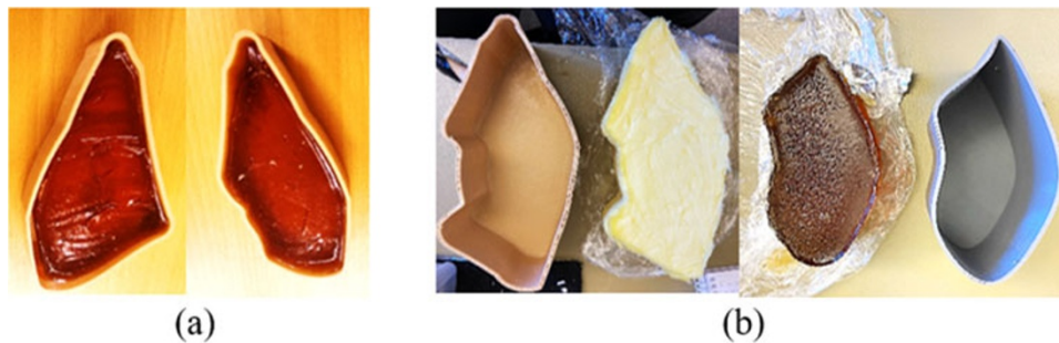
Figure 4. (a) Fabricated left and right lobes of healthy deflated lung TEMs and (b) molds together with inflated and deflated left lobes of healthy lung TEMs.
