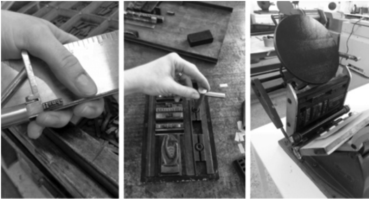
Figure 2 The process of setting type and printing on an Adana tabletop press. Photograph by and of the author, 2014.
