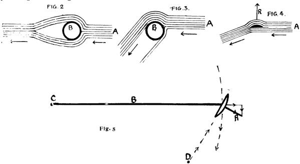
the original stream. The reaction can be represented by a line R at right angles to the flat face (this is approximately correct), and we now have the clue to the behaviour of the ball.
