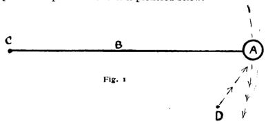
The diagram (fig. 1) shows in plan the necessary apparatus. The ball A is supported by a rod B which is supported in its turn at axis C, round which it is free to swing in a horizontal plane. The demonstrator causes the ball to travel towards him by blowing on it from point D.
