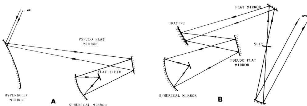
Figure 2. Optical lay-out of the two modes : a) photometric mode ; b) spectrographic mode.
