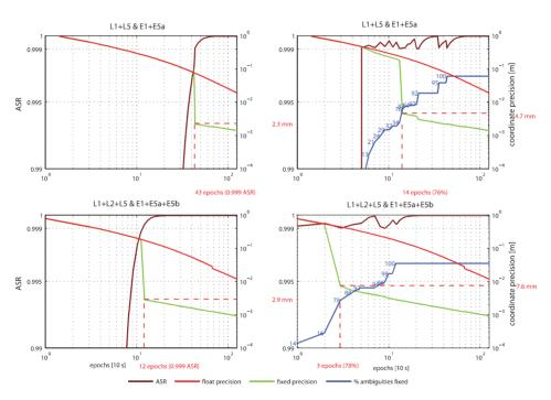
Figure 5. GPS+Galileo ambiguity success rates (ASR) and coordinate precision vs. number of epochs, for: L1+L5 & E1+E5a (top) and L1+L2+L5 & E1+E5a+E5b (bottom), for a data sampling interval of 10 s. The left graphs relate to FAR, while the right graphs relate to PAR, both based on the criterion that ASR  $\ge 0.999$ . See Figure 2 for an explanation of the different curves.
