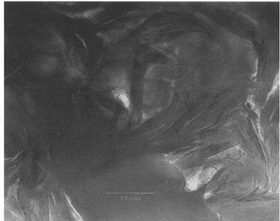
Figure 7. TEM showing wavy smectite-like clays (possibly smectite, possibly with some illite) growing out from corroded glass (even contrast area at bottom center) surfaces in sample GU3 1406.
