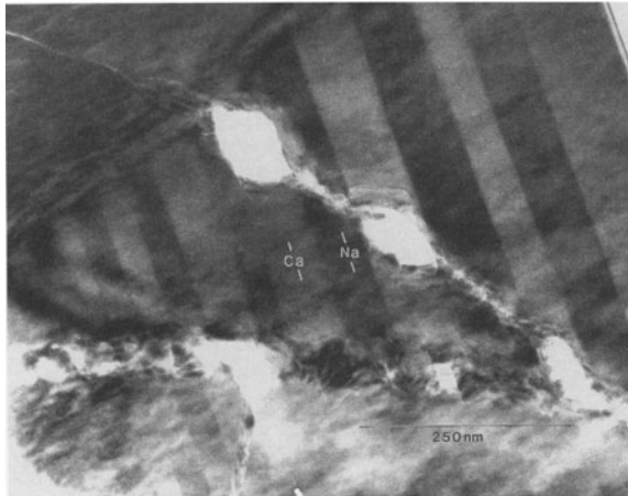
Figure 17. TEM illustrating dissolution features in groundmass feldspars in G4 272. Alkali feldspar (top left) shows no alteration. Exsolution lamellae in plagioclase that are richer in Ca (light contrast, labelled "Ca") show significant dissolution focused at crack surfaces compared to albite-rich lamellae (labelled "Na").
