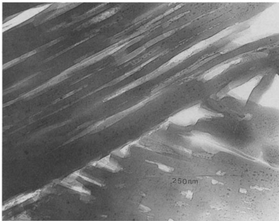
Figure 1. a) TEM of sample G4 1531 showing an apparent continuum from etched glass to crystalline elongate zeolites. b) Area similar to (a) at higher magnification. Note the large amount of <50-nm-diameter porosity.
