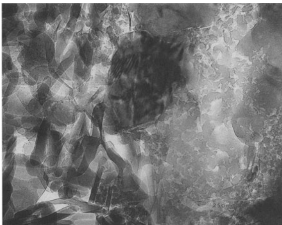
Figure 6. TEM of glass (top right), zeolites (tabular crystals mostly on the left), opal-like silica and etched glass (center and right). A small, twinned, essentially unweathered crystal of K-feldspar (dark contrast center top) is shown (sample G4 1531).
