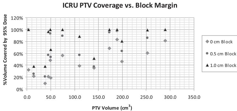
Figure 4. Plot of percentage PTV volume covered by 95% of the prescription dose as a function of block margin for all of the ICRU normalised cases. Trend lines are drawn to help guide the eye.
