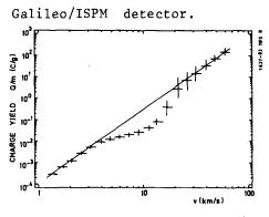
Figure 2. Charge yield Q/m (ions) plotted against velocity. In the region between 4 km/s and 20 km/s Q/m shows a deviation from a power law, fitted at low and high velocities.
