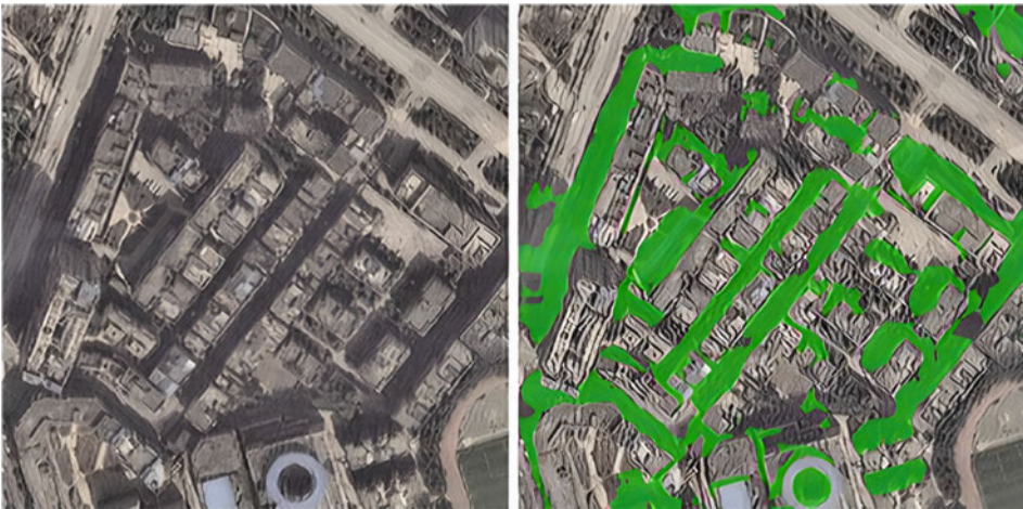
Figure 19. Application of data collected by satellites to monitor construction rate using segmentation [92].
