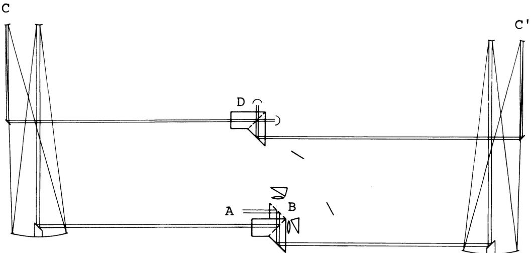
Figure 3. Full-aperture metrology. Optical paths shown are for the metrology signal only.
