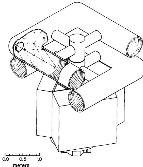
Figure 1. An artist's rendition of a Mini-POINTS with 2 m separations between pairs of 25 cm telescopes. The instrument comprises two U-shaped interferometers joined by a bearing which permits  $\phi$ , the angle between the principal axes of the interferometers, to vary from its nominal of  $90^\circ$ . The Multimission Modular Spacecraft is shown mounted under the instrument.
