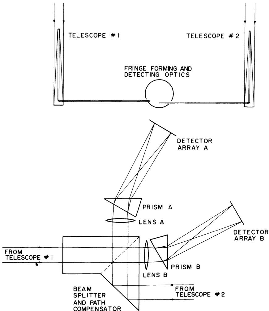
Figure 2. Optical design. Top: general scheme. Bottom: fringe forming and detecting optics.
