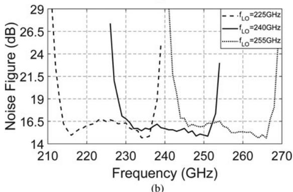
Fig. 11. Measured channel bandwidth (a) and NF (b) of the receiver for different carrier frequencies.
