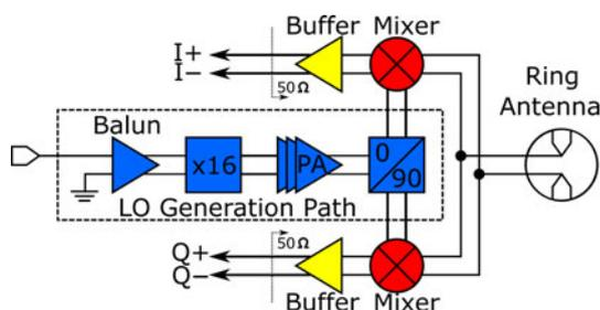
Fig. 1. Block diagram of the IQ direct-conversion mixer-first receiver.
