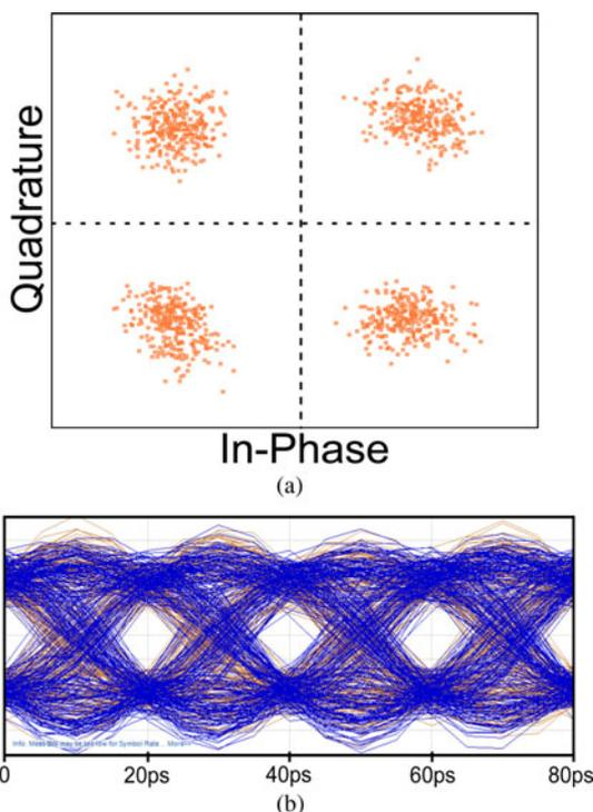
Fig. 13. Constellation (a) and eye diagram (b) for 50 Gbps QPSK working at a carrier frequency of 240 GHz (EVM=19%).
