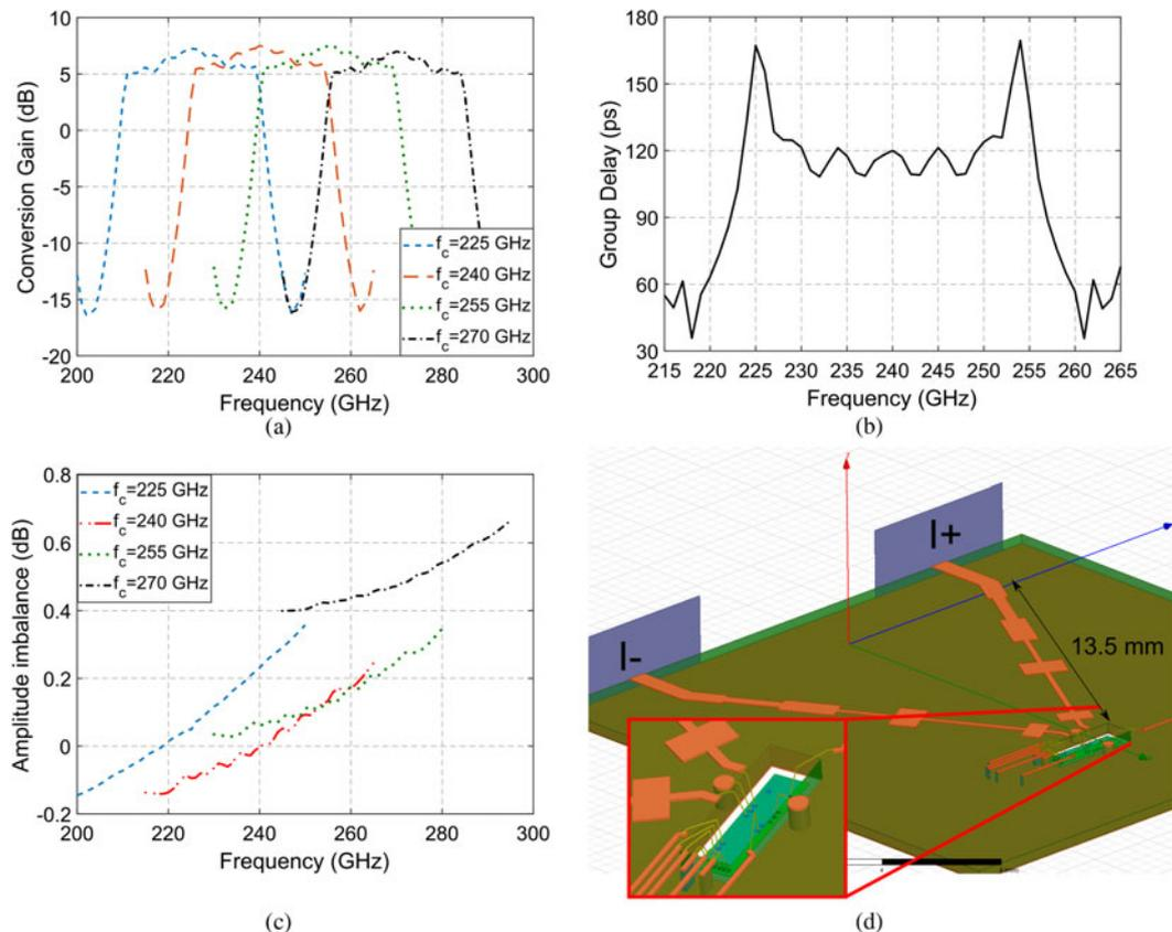
Fig. 6. Simulated receiver RF/IF BW for IQ channels combined at different carrier frequencies (a), group delay (b), IQ amplitude imbalance, (c) and 3-D model of the IF filter. (d) The 3-dB BW is 28 GHz, independently of the carrier frequency, with in-band ripples under 1 dB. The group delay is only plotted for a carrier frequency of 240 GHz. It is similar at other carrier frequencies, with variations under 1% for different carriers. The amplitude imbalance stays below 0.7 dB.
