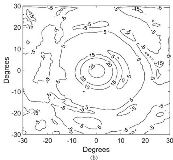
**Fig. 9.** Antenna directivity for the frequency band (a) and measured azimuthal view of the radiation pattern at 240 GHz (b).
