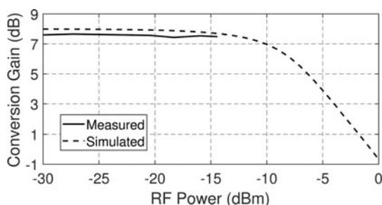
Fig. 12. Linearity of the receiver. The simulated  $P_{1\text{ dB}}$  is  $-10$  dBm at 240 GHz. Due to the free-space setup, the maximum power available at the input of the receiver is  $-14.5$  dBm. Therefore, the  $P_{1\text{ dB}}$  was not reached in the measurements.
