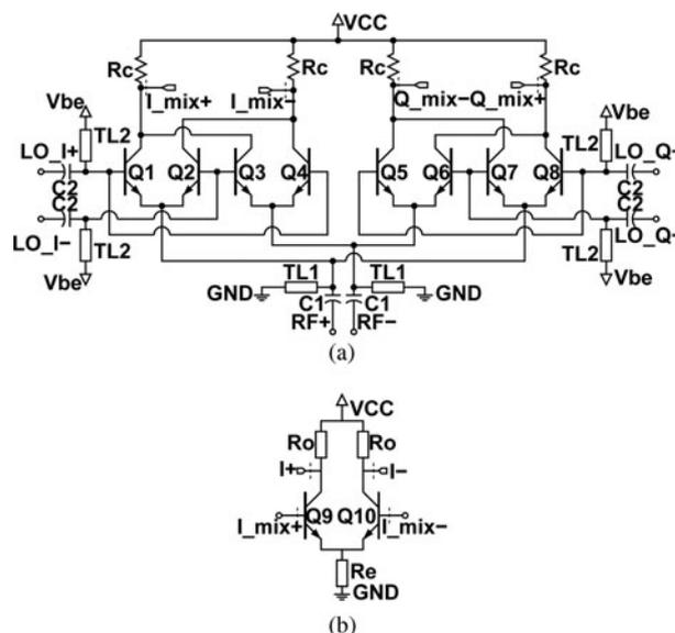
Fig. 2. Schematic of the quadrature direct-conversion mixer (a) and one of the output IF buffer (b).
