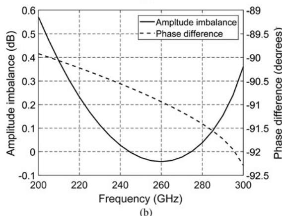
Fig. 4. Simulated power at the output of the PA and the hybrid (a) and amplitude-imbalance and phase difference (b) at the output of the hybrid.
