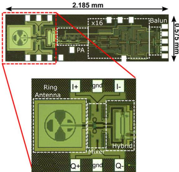
Fig. 5. Chip micrograph of the receiver.
