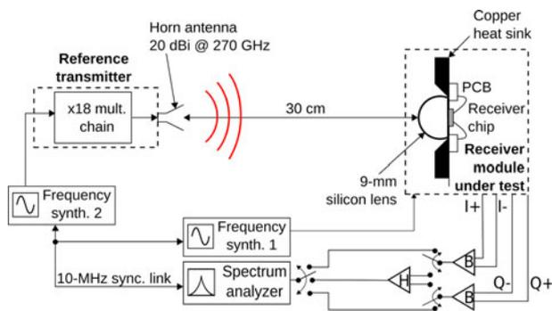
**Fig. 8.** Free-space characterization setup of the receiver. The differential output signals were combined with baluns (B) and a hybrid (H) was used for the SSB NF measurement.
