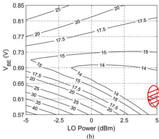
Fig. 3. Contour plot of the CG (a) and NF (b) for both IQ channels combined versus LO power at the input of the hybrid and the mixer  $V_{BE}$ . The operating region is marked in red.
