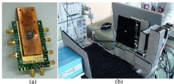
**Fig. 7.** Receiver module (a) and picture of the measurement setup (b) The chip is fixed to the lens with epoxy and assembled on a broadband PCB. The set up is completely covered by absorbers to reduce the impact of reflections.
