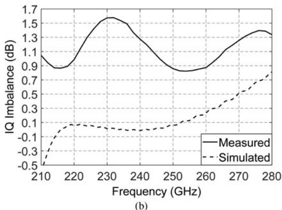
Fig. 10. Receiver CG, NF (a) and IQ imbalance (b) This measurement was performed for a fixed IF of 33 MHz.
