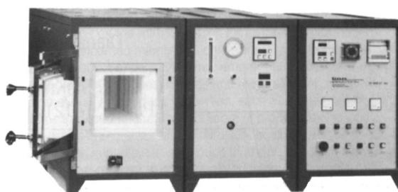
**High temperature furnace HT** for universal heat treatment and sintering under air, gas and vacuum, short heating and cooling cycles, ceramic fibre or Graphite felt insulation, 1400 °C – 1900 °C, chamber volumes 4 to 52 liters; special systems on request.
