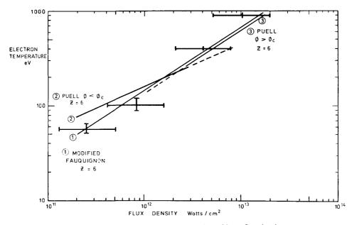
Fig. 2. Electron temperature as function of laser flux density.
