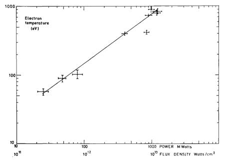
Fig. 1. Electron temperature as function of laser power (flux density values approximate).
