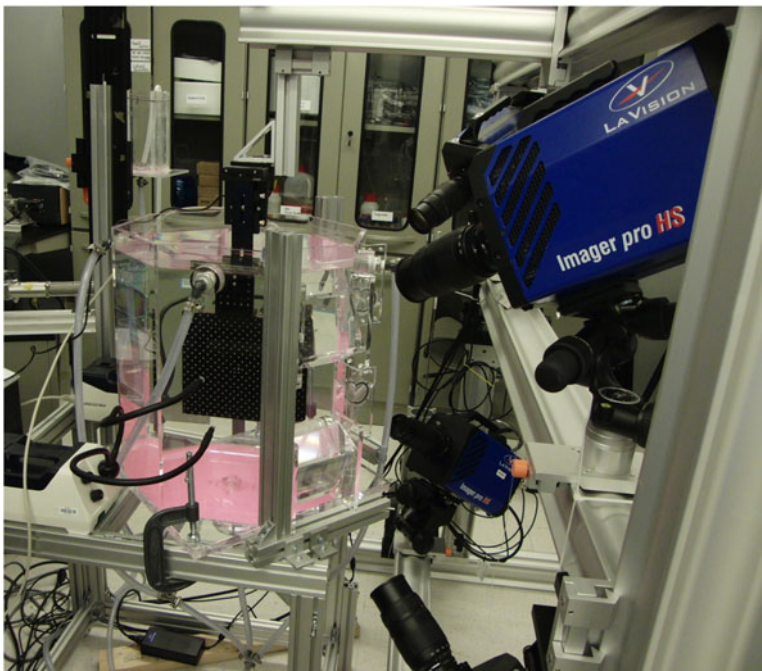
Figure 20. Photograph of the experimental set-up with the camera arrangement. The calibration plate is moved in the measurement region inside the octagonal tank using a motorised linear traverse. The four high-speed video cameras are focused on the measurement region with lenses mounted on Scheimpflug attachments. Two water-filled prisms, visible on the right-hand side of the tank, are implemented to minimise optical distortions.
