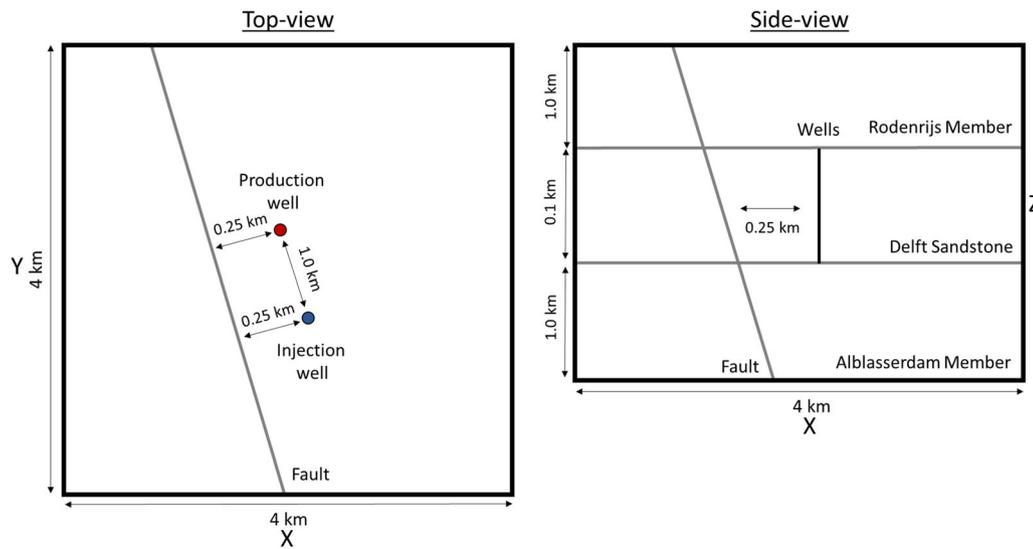
**Figure 3.** Top (left) and side (right) view of the Delft sandstone model (not to scale).
