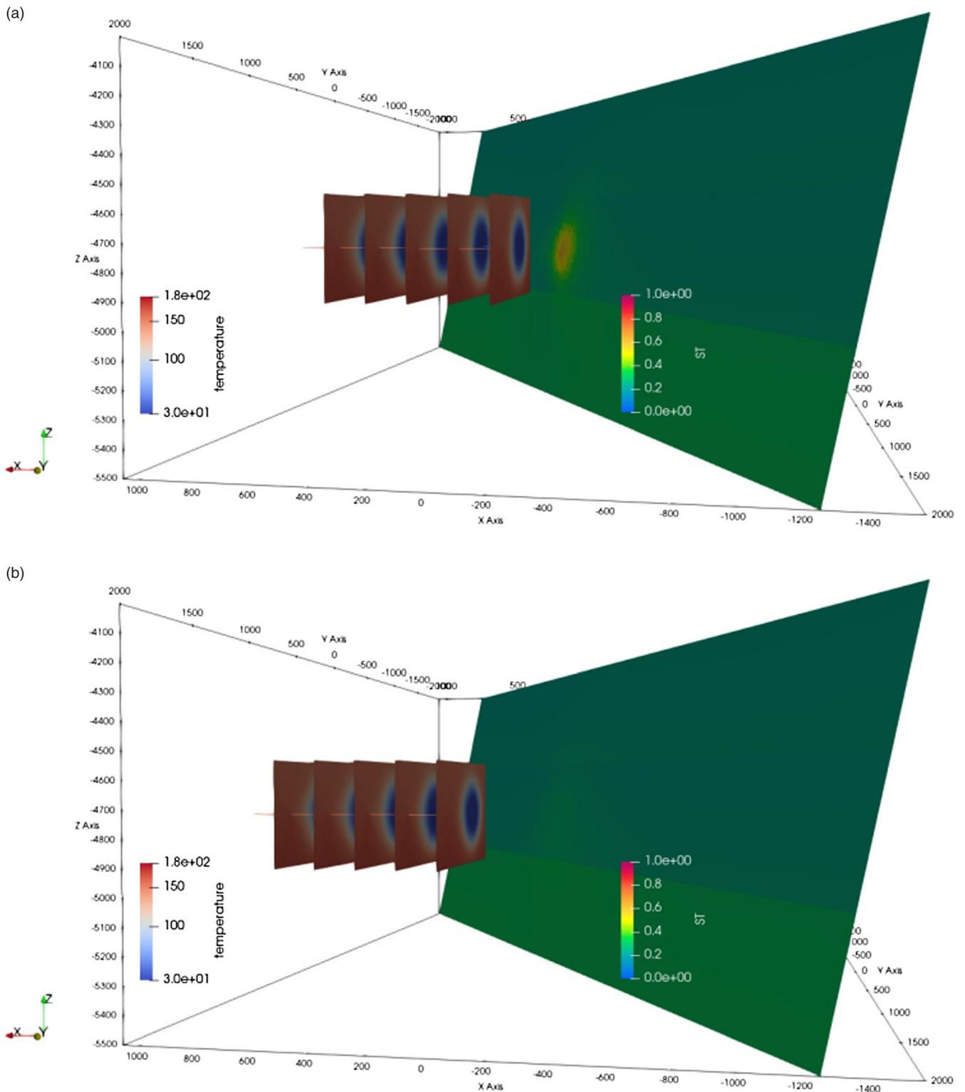
**Figure 16.** Comparison of temperature distribution on hydraulic fractures and slip tendency on the fault after 30 years of circulation in (a) the Dinantian EGS model with 250 m well-fault spacing and (b) 500 m well-fault spacing.
