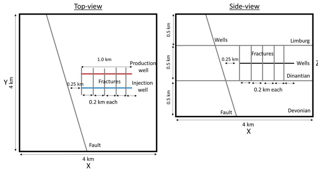
**Figure 6.** Top (left) and side (right) view of the Dinantian EGS model (not to scale).
