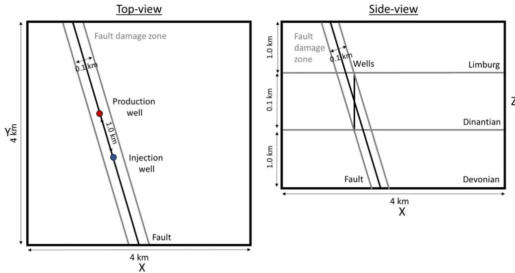
**Figure 5.** Top (left) and side (right) view of the Dinantian fault damage zone model (not to scale).
