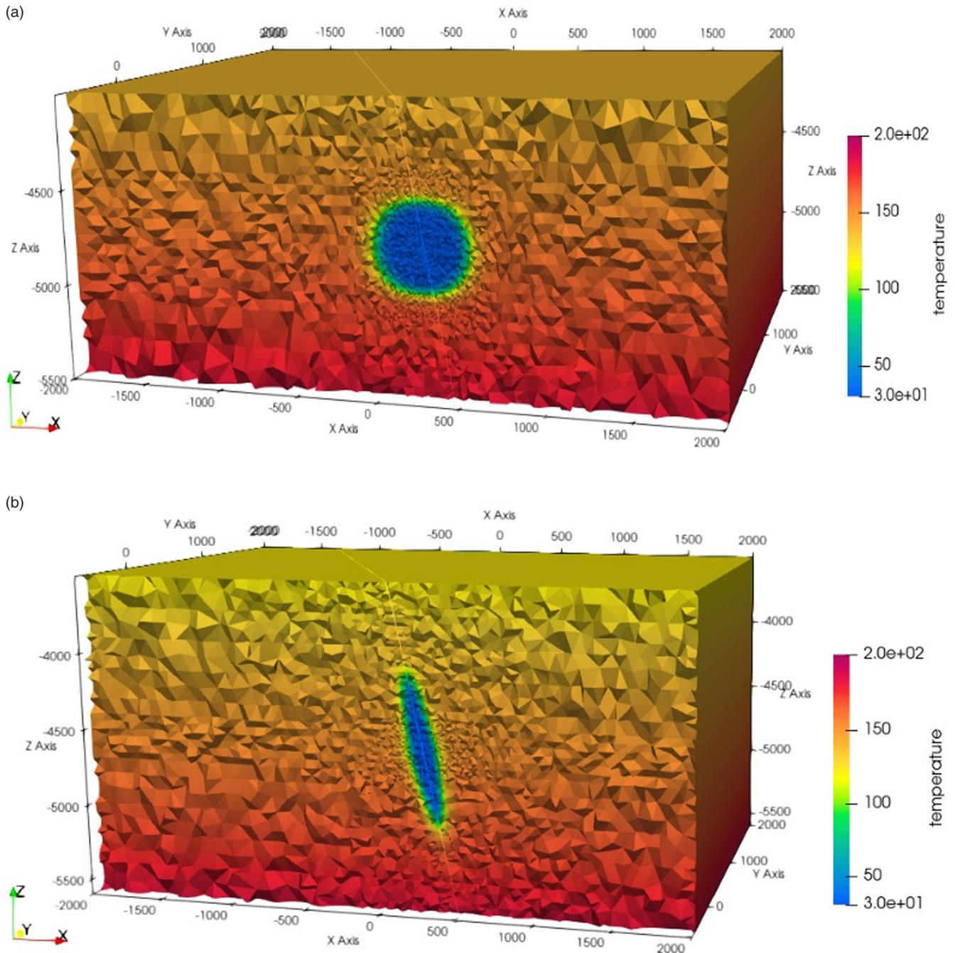
**Figure 15.** Comparison of temperature distribution after 30 years of circulation in the (a) Dinantian fault model and (b) the Dinantian damage zone model.
