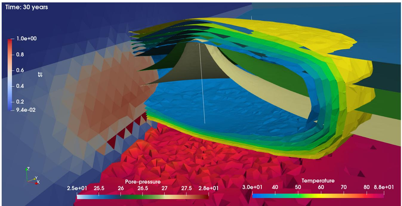
Figure 8. Temperature contours (in °C), pressure contours (in MPa) and slip tendency (unitless) on the fault in the Slochteren base case model after 30 years of circulation.
