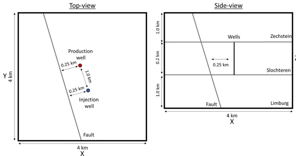
**Figure 1.** Top view (top left) and side view (top right) for the Slochteren base case model (not to scale).
