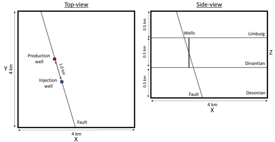
**Figure 4.** Top (left) and side (right) view of the Dinantian limestone fault model (not to scale).
