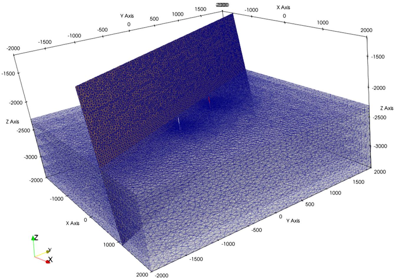
**Figure 2.** 3D view of the Slochteren base case mesh. Mesh refinement is applied around the injection and production wells and in the fault plane within the reservoir unit.
