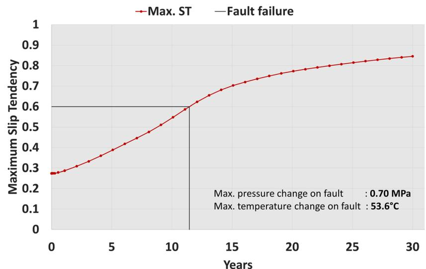
**Figure 7.** Maximum slip tendency on the fault and fault failure within the reservoir unit of the Slochteren base case model.
