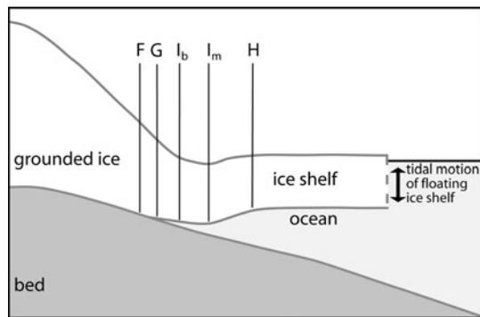
**Fig. 1.** Schematic diagram showing the key features of a typical ice-shelf GZ, based on Smith (1991), Vaughan (1994) and Fricker and others (2009). Point F is the landward limit of ice flexure from tidal movement; point G is the true GL where the grounded ice first loses contact with the bed; point  $I_b$  is the break-in-slope; point  $I_m$  is the local minimum in topography; and point H is the hydrostatic point where the ice first reaches approximate hydrostatic equilibrium.
