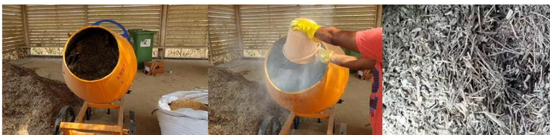
Figure 3: Preparing the Bio-Bricks mixture
