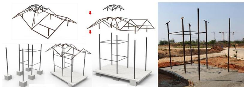
Figure 5: Frame structure for prototyping
