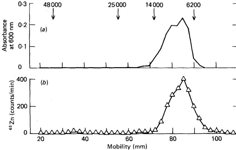
Fig. 4. Sodium dodecyl sulphate electrophoresis of the copper-zinc material (fraction 4, Table 2) separated after incubation of lipid-protein aggregate and Sephadex G-50 and DEAE-cellulose chromatography from an animal injected with  $^{65}\text{Zn}$ . (a), The gel scan after staining; (b),  $^{65}\text{Zn}$  following slicing. ↓, Molecular weights indicated.
