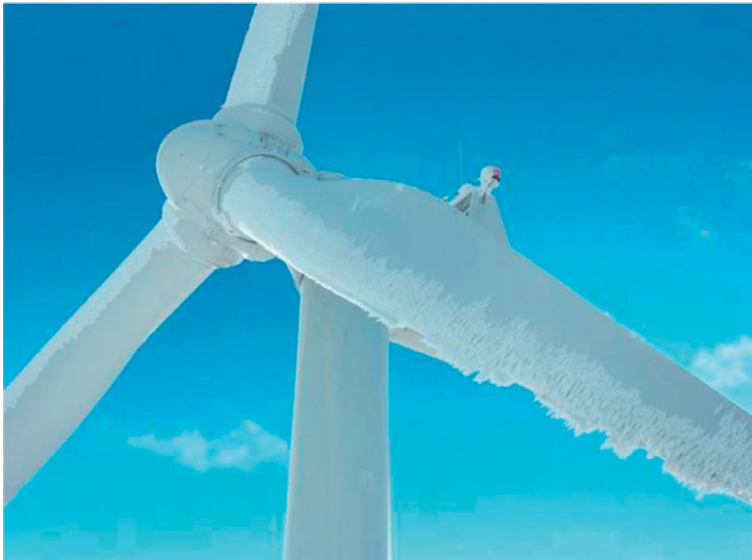
Figure 1.2 Icing on a wind turbine blade caused by impact of freezing rain or drizzle (Larsen, 2021).
