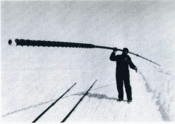
Fig. 2. PICO driller with 9 m of extensions and 2 m auger barrel.
