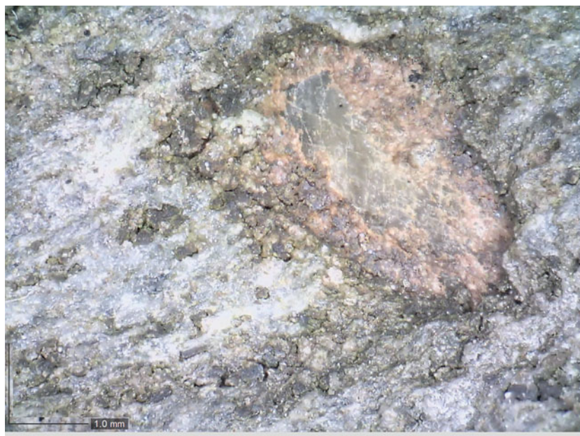
Figure 15. High magnification of a decayed mineral through chemical dissolution and leaching of iron from within the rock matrix of Dunchraigaig capstone. (Photograph: Callum Graham.)
