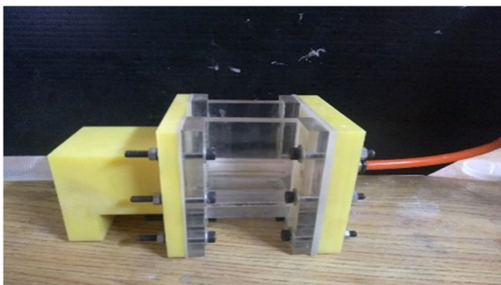
Fig. 13 Apparatus used to determine the permeability of a wick structure
