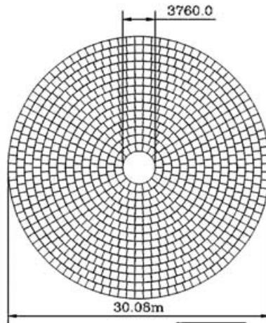
**Figure 8.** JELT segment configuration. A total of 798 segments, about  $1\text{m} \times 1\text{m}$  in size, are configured in 14 concentric rings to form a 30m mirror. Note that in this configuration, we need only 14 different aspheric shapes in contrast to the 123 different hexagon shapes required for the 738 segment concept of the TMT.
