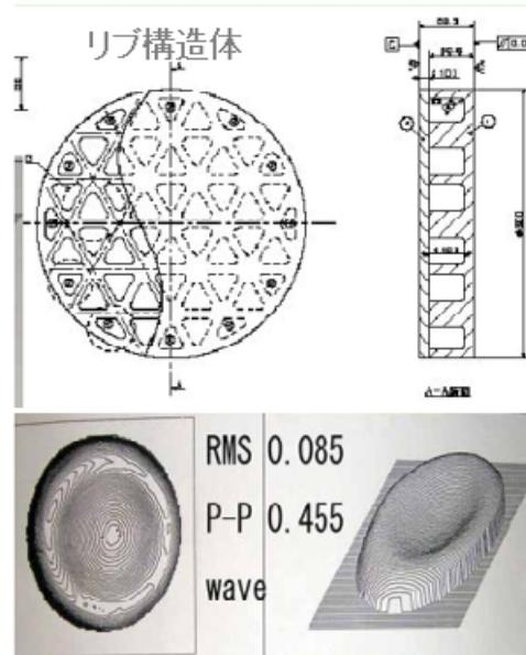
**Figure 6.** Light weight structure of a 30cm spherical ZPF mirror and its error figure.
