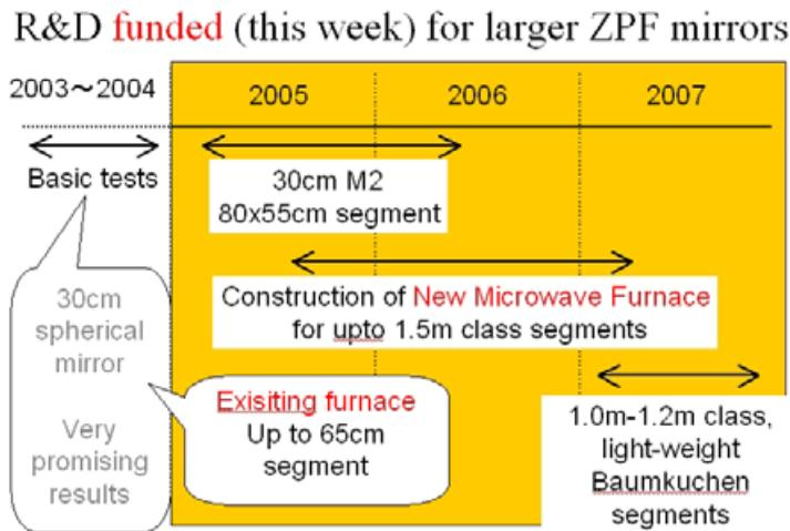
**Figure 7.** Schedule for manufacturing a new microwave furnace to sinter larger ZPF blanks.
