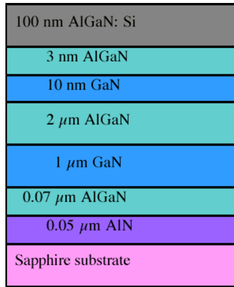
Figure 1. Growth structure of the modulation doped quantum well sample.
