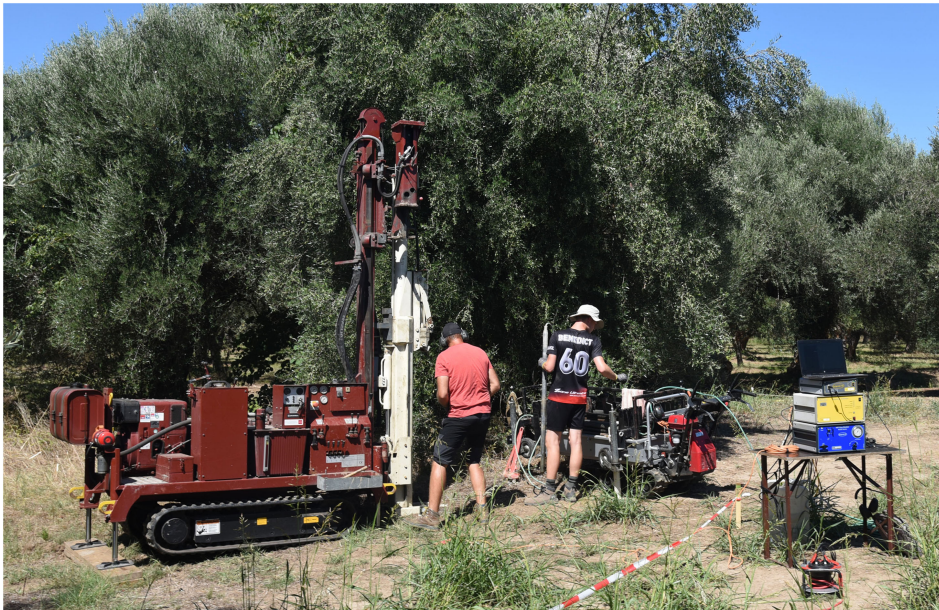
Fig. 3.42. Olympia: ge archaeological direct push soundings and boreholes south of the Southwest Baths. © DAI.
