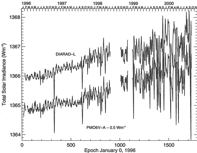
Figure 2. Time-series of the level-1 observations of PMO6V and DIARAD, after correction of their exposure dependent changes.
