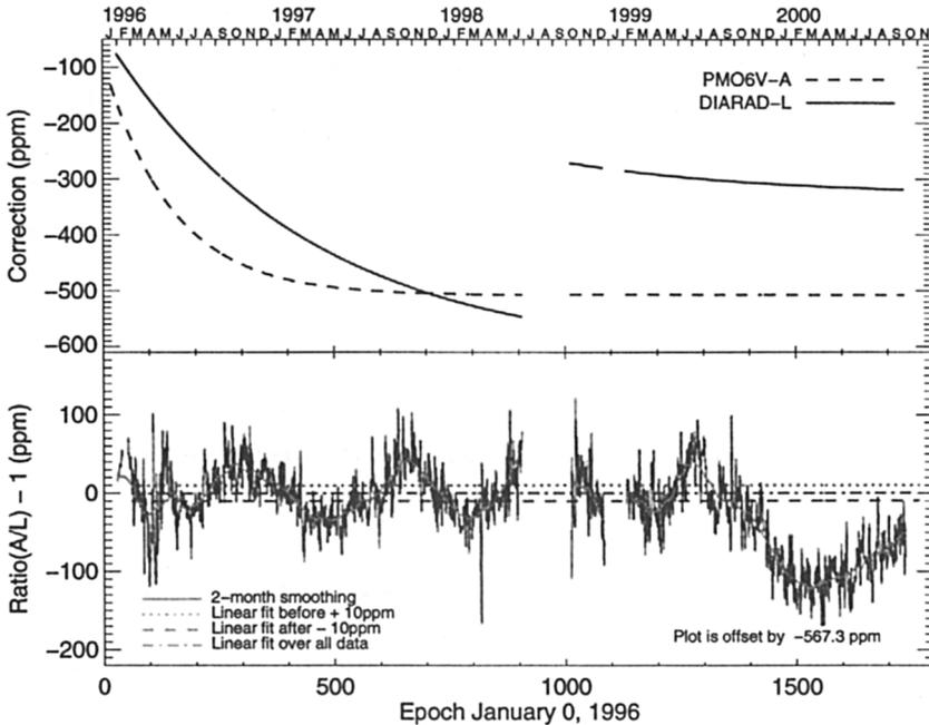
Figure 3. Corrections for the exposure independent behaviour of PMO6V-A and DIARAD-L (top panel) and the corrected ratio (lower panel).
