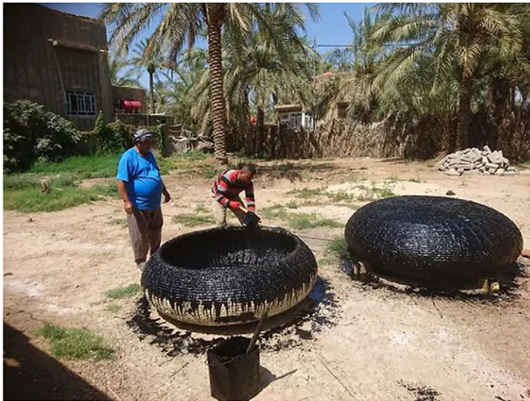
Figure 13. Pitch being applied during the reconstruction of traditional Guffa coracles by Safina Projects in Hilla, Iraq, May 2018. © Rashad Salim. Used with permission.
