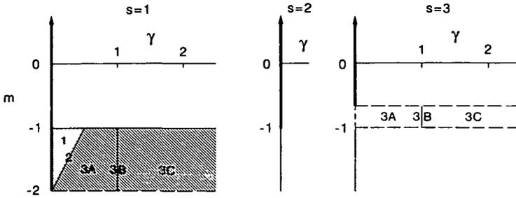
FIGURE 3. Maps of the  $(\gamma, m)$  plane for  $s = 1, 2, 3$ , showing regions giving similarity solutions of the various types, classes, and subclasses. See text for explanation of material-losing solutions with  $s = 3$ . The bold lines along (part of)  $\gamma = 0$  represent the material-preserving solutions.
