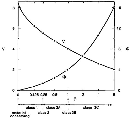
FIGURE 5. Integral properties of solutions for  $s = 1, m = -\frac{3}{2}$ . Reduced slug magnitude  $V$  and reduced flux at infinity  $\Phi$  as functions of  $\gamma$ . Dots indicate the calculated points. The scale of the abscissa is linear in  $\ln(\gamma + 0.125)$ .
