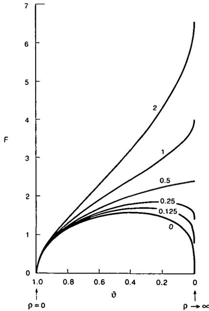
FIGURE 6. Flux-concentration relations for  $s = 1, m = -\frac{3}{2}$ . Reduced flux  $F$  as a function of  $\vartheta$  for the indicated values of  $\gamma$ .
