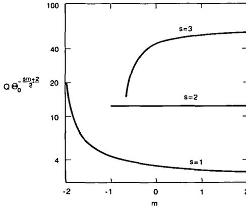
FIGURE 2. Material-conserving instantaneous sources. Slug magnitude in the reduced form  $Q\Theta_0^{(sm+2)/2}$  as a function of  $m$  for the indicated values of  $s$ .
