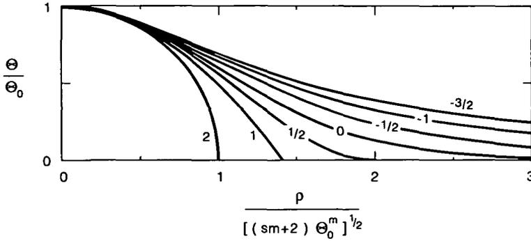
FIGURE 1. The material-conserving instantaneous source solutions in the reduced form  $\Theta/\Theta_0$  as a function of  $\rho [(sm + 2)\Theta_0^m]^{-1/2}$ . Numerals on the curves are values of  $m$ .
