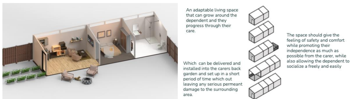
Figure 2. An illustration of the final design (left) and possible construction options (right)
