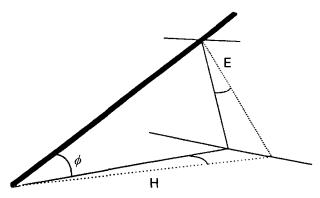
FIGURE 2. To calculate hour angles, H, for a horizontal surface use tan H =  $\sin \phi$  tan E where  $\phi$  is the latitude of the location and E the hour angles on the equatorial plane. (For vertical dial angles simply replace by the colatitude, 90  $\phi$ .)
