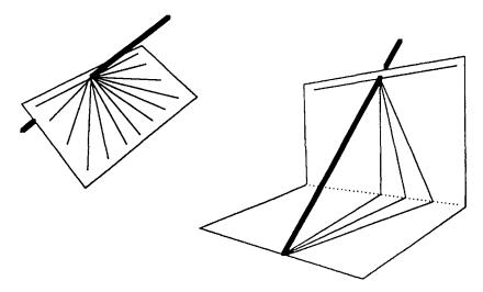
FIGURE 1. Sketches showing the equatorial model and the vertical and horizontal planes. Combining the two together reveals the relationship between hour lines on all surfaces.
