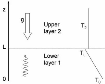
**Figure 1.** Two-layer model depicting a stratified solar atmosphere. The lower part of the atmosphere (index 1) is separated from the upper part (index 2) by a density and temperature discontinuity at  $z = L$ . Waves are launched at  $z = 0$  and propagate in the vertical  $z$ -direction.
