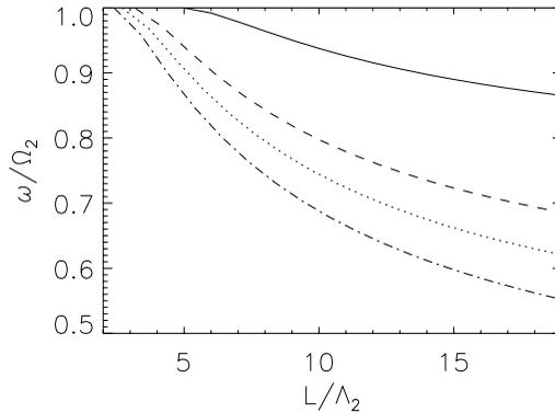
**Figure 2.** Scaled resonant frequency  $\omega$  as a function of the length of the non-uniform layer  $L$ . Four different cases are shown:  $T_0/T_2 = 2$  (solid line),  $T_0/T_2 = 5$  (dashed line),  $T_0/T_2 = 8$  (dotted line) and  $T_0/T_2 = 15$  (dash-dotted line). In all four cases,  $T_L = T_2$  is set.
