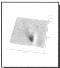
**AFM/ PicoIndenter** from Hysitron works with your AFM to provide imaging, positioning and light load nN resolution for nano-scale films and surfaces. Picture shows picoindent on silicon wafer
