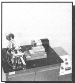
**Universal Wear Machine** from Biceri provides three test modes to simulate the rotary, sliding wear and lubrication conditions found in all kinds machinery.
