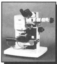
**Diamond Stylus Scratch Tester** The classic Revetest and Micro Scratch testers from CSEM use acoustic emission detection for characterizing the adhesion of coatings.
