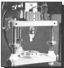
**3D Profilometer** from Scantron uses laser triangulation to map extremely fine displacements of surface features or texture. Largest measuring range of any such equipment.
