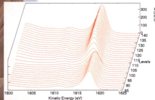
*Using high energy resolution, the MICROLAB 310F can distinguish chemical states. In this depth profile of TiSi on Si, the change in the chemical state of Si can be seen at the interface.*
