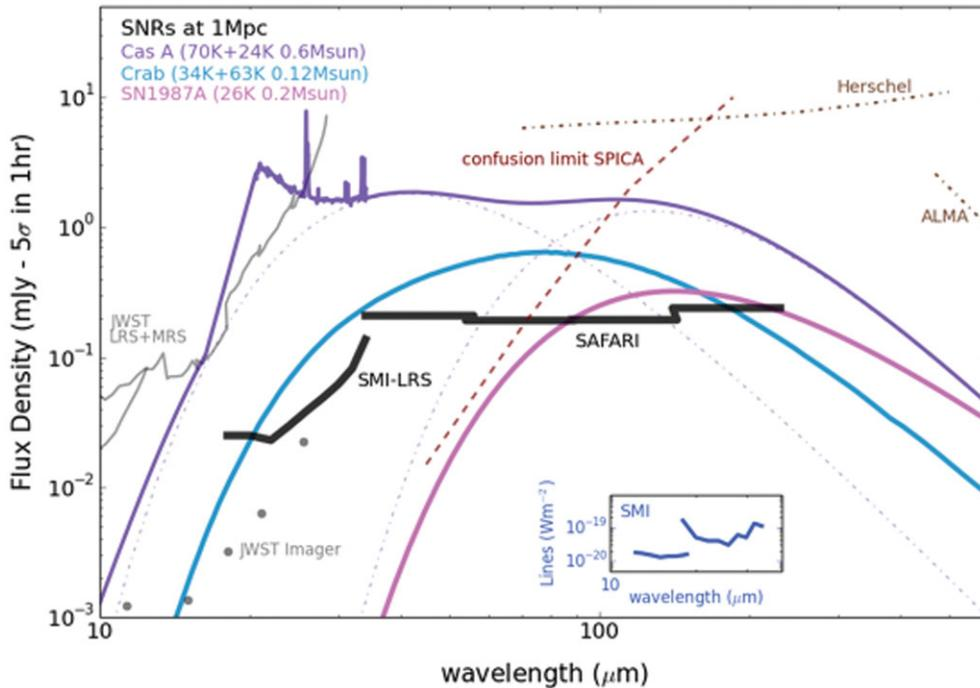
**Figure 8.** Sensitivity comparison for *SPICA* SAFARI and SMI (solid black lines) compared to *Herschel*, ALMA, and *JWST* in dot-dashed grey. The inset shows the  $5\text{-}\sigma$ , 1 h levels, line sensitivities for *SPICA* SMI MRS and HRS spectrometers. The confusion limit is shown as a dashed line.
