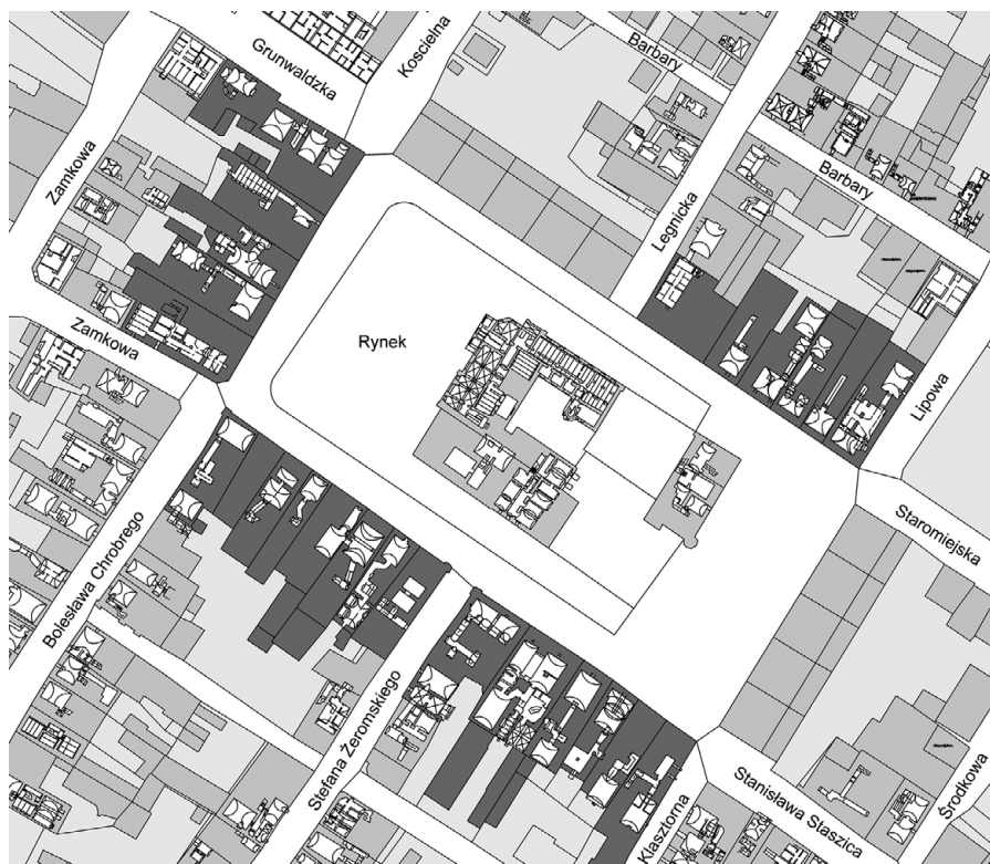
Figure 13. Jawor, plan showing the layout of the cellars under the arcaded houses standing at the market square (marked with dark grey).
