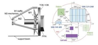
**Figure 6.** Left: Configuration of the *SPICA* telescope assembly. The scientific instruments are mounted in Focal Plane Instrument Assembly (FPIA), on the optical bench on the rear of the telescope. Right: The *SPICA* instrument focal plane layout.
