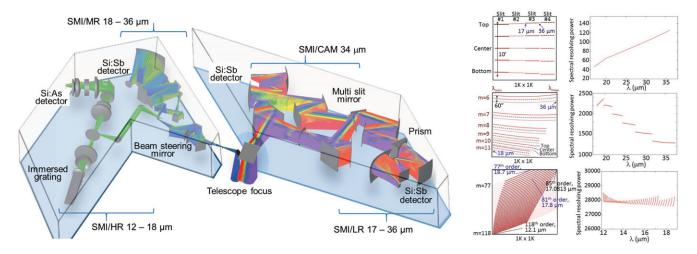
Figure 15. Left: optical layout for SMI/MR–HR and SMI/LR with SMI/CAM. The colour coding of rays is based on the angular positions in the fields-of-view. Right: Spectral formats and spectral resolutions of SMI/LR, SMI/MR, and SMI/HR (top to bottom).
