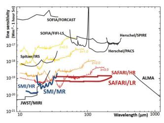
**Figure 4.** Projected spectroscopic sensitivity of the *SPICA* instruments as compared to other infrared facilities (at the SAFARI/LR resolution of  $\sim$ 300). The SAFARI sensitivity assumes a detector NEP of 2  $\times$  10<sup>-19</sup> W  $\sqrt{\rm Hz^{-1}}$ . The infrared spectrum of the Circinus galaxy, scaled to  $L=10^{12}~\rm L_{\odot}$ , for redshifts 0.5 to 3, and smoothed to the SAFARI/LR resolution, is superimposed.
