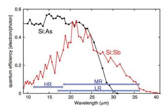
**Figure 16.** Quantum efficiency for Si:As (*JWST*/MIRI; Ressler et al. 2008) and Si:Sb (test model for SMI; Khalap et al. 2012) arrays that are currently available. The SMI wavelength range is shown in blue.
