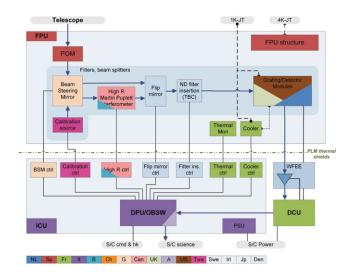
**Figure 10.** The functional block diagram for SAFARI. The top part represents the focal plane unit mounted on the 4.8-K instrument optical bench. The bottom part shows the warm electronics, mounted on the CRYO assembly.
