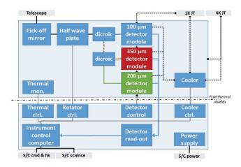
**Figure 17.** POL functional block diagram, implementing individual direction of three wavelength bands onto a common focal plane assembly. An achromatic half-wave plate in the common part of the optics train is used by all bands.
