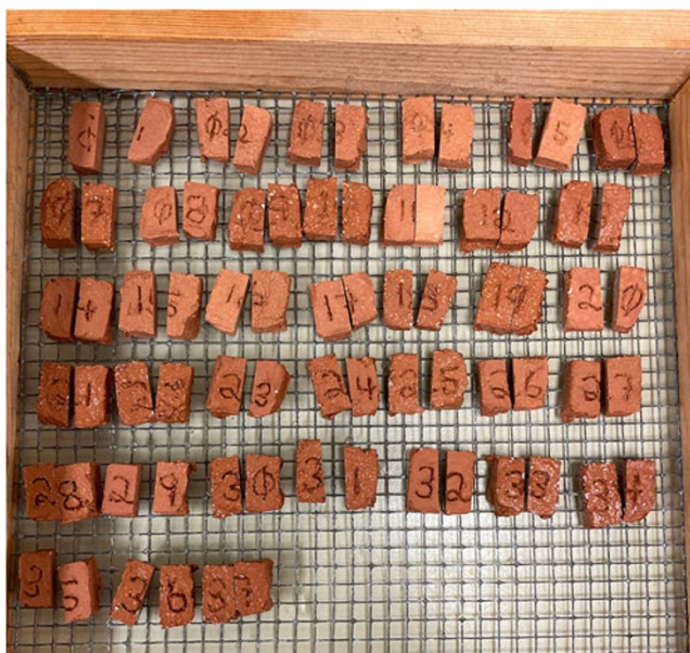
Figure 4. First 37 briquettes after firing, sawn in half (photograph by Lindsay C. Bloch).
