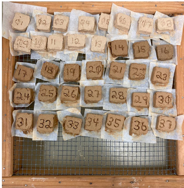
Figure 3. Batch of briquettes drying. The first 13 paler briquettes are bone dry, while 14–37 are still wet (photograph by Lindsay C. Bloch).
