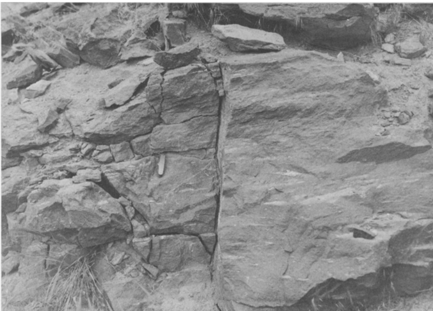
Fig. 5. Joint spacing in nearly fresh basaltic andesite at northeast entrance to silica pit (knife about 5 in. long).
